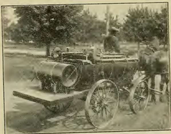
FIG. 1.—Invincible Mounted Sprayer—Wallace Machinery Co. The spray liquid is pumped into an airtight tank together with compressed air by pumps driven from the wheels. When machine is standing still the compressed air continues the work.
