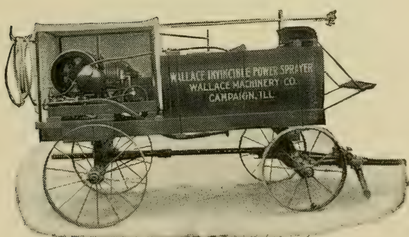
FIG. 2.—Gasolene power sprayer with air-cooled engine. PLATE XIV.
