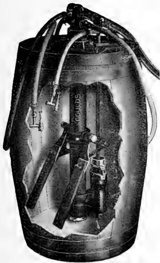
FIG. 1.—Barrel pump showing agitator.
