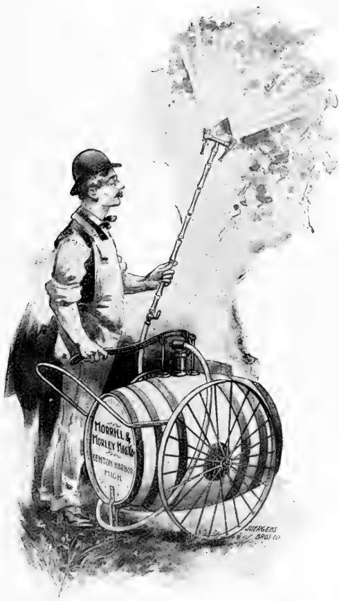
PLATE XI.—Small portable barrel pump. See page 67.
