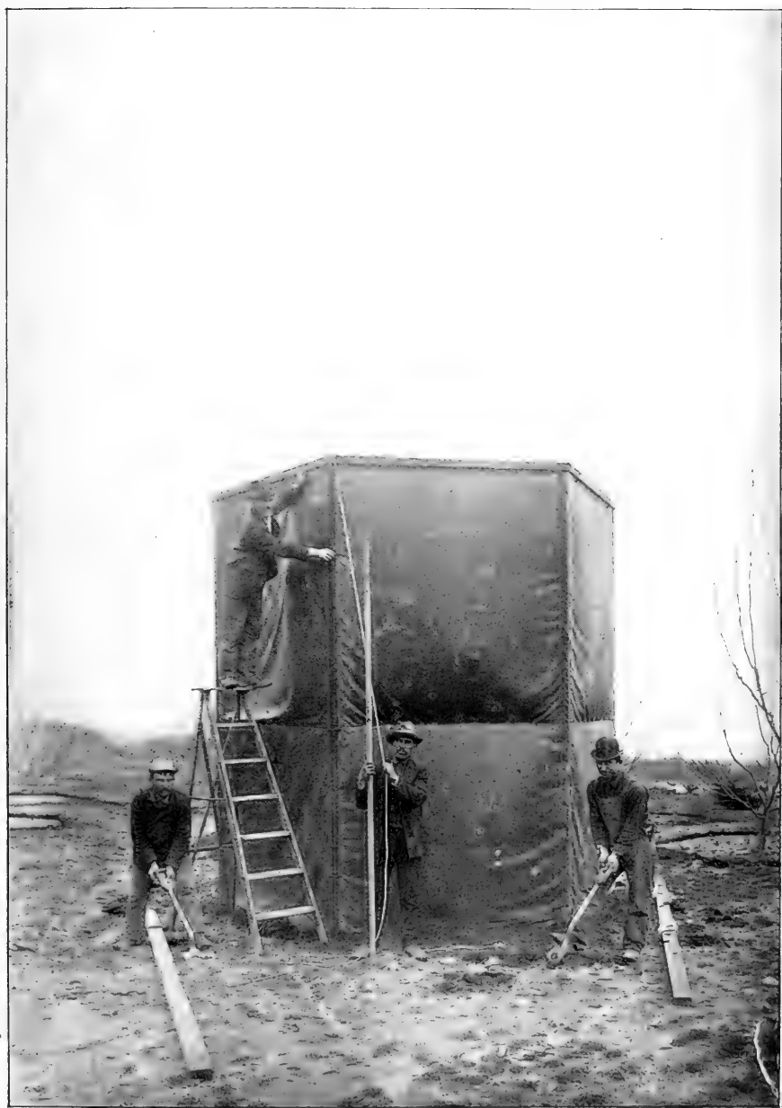
PLATE XVII.—Hexagonal Fumigator for trees. This fumigator is made in sections and is taken apart in moving. For explanation see page 76.
