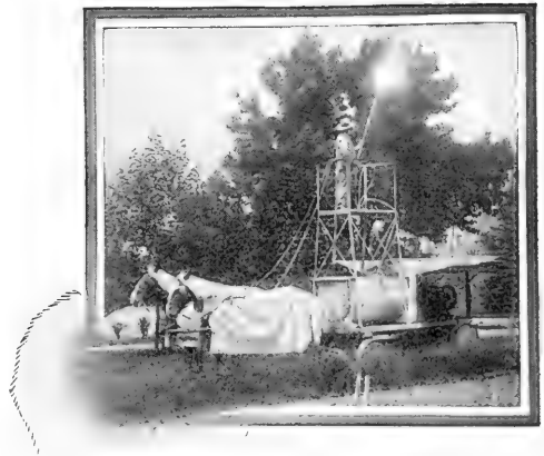
FIG. 4.—Gasolene power sprayer in operation.
