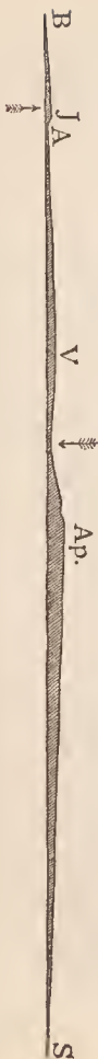
Fig. 6.—Section from Basle across the Alps to Senago, north-west of Milan. B , Basle. J , Jura. A , Aar, near Olten. Ap , Alps. S , Senago. Inclination from Basle to summit of Jura, 1^{\circ} 37' ; from Basle to the summit of the Alps, 1^{\circ} 43' .
