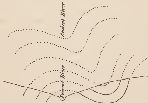
FIG. 57.—Diagram to illustrate a river now running in an anticlinal.
