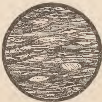
FIG. 21.—Section of a similar rock which has been compressed, and in which cleavage structure has been developed.
