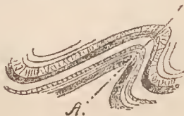
FIG. 12.—An Inclined Fold.
