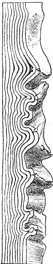
FIG. 4.—Showing the artificial folds produced in a series of layers of clay on indiarubber, according to an experiment by Prof. A. Favre.
