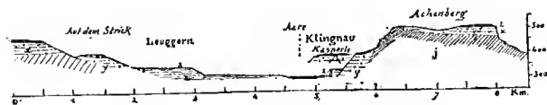
FIG. 34.—Section across the Valley of the Aar above Coblenz. Scale, length 1=100,000; height 1=25,000. z, Lower alluvial terrace; y, upper alluvium covered by moraines and Löss; x, alluvium of the upper plateaux, covered by Löss; Jurassic strata in situ .
