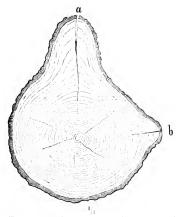
Fig. 239. Transverse section of an oak with two trosteracks, a and b.
