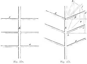
Plans of drainage. h. Main-drain. s. Feeders.
