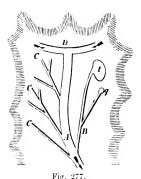
D. Chief feeder. A. Main drain. B. Leader from a spring q, and a small swamp t. C. Feeders.
