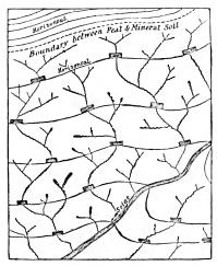
Fig. 279.—Kaiser's method of drainage.
