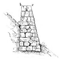
Fig. 282.—Dry masoury wall for protection against avalanches.
