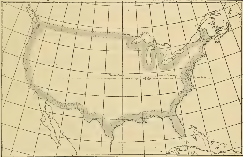
Transverse polyconic Projection of the United States Drawn by A. K. Eastman.
