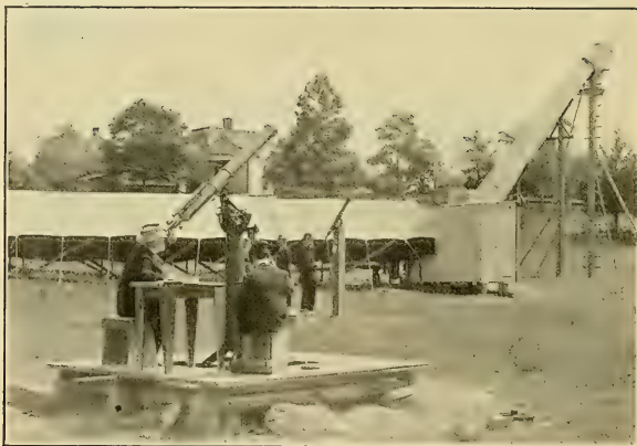
FIG. 4. Dark room and tubes of 135 foot and 38-foot telescopes. 5-inch equatorial in foreground, Professor Langley observing.
