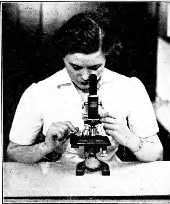
Fig. 6.—Correct position when using a microscope. The microscope should stand upright on the table directly in front of the observer. The left hand should be used on the fine adjustment to maintain the proper focus, thus leaving the right hand for other work while looking through the eyepiece. Both eyes should be kept open in order to minimize eyestrain. This microscope has three objectives on the nosepiece and a mechanical stage to move the slide on the stage. (From Carter: Microbiology and Pathology , The C. V. Mosby Co.)
