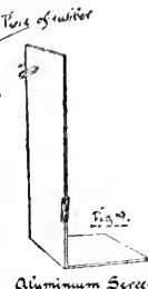
Aluminum Screen with clips for holding ends. Section shows automatic grip of piece of rubber.
