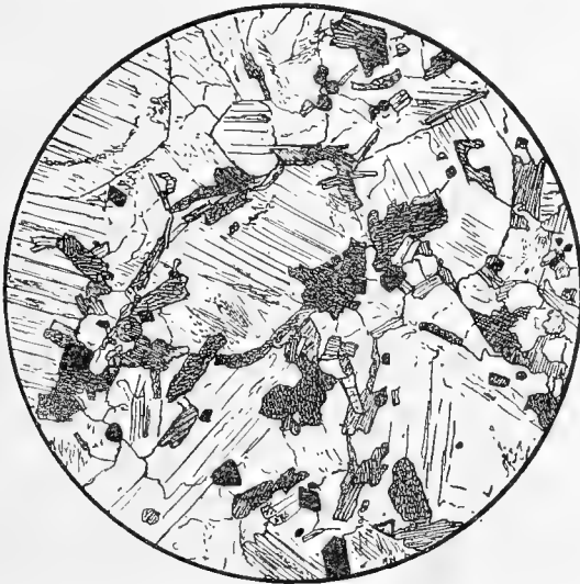
FIG. 2.—Thin section of central portion of spherulite from granite of Mullaghderg, showing arrangement of biotite, which represents the residue of an inclusion, around crystals of felspar. \times 14 . Geological Survey specimen.
