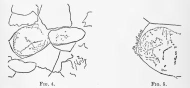
FIGS. 4 and 5.—Section of quartzite from near Amlych, showing secondary growth of quartz on rounded grains. FIG. 5.—Somewhat more highly magnified (the striæ on the left-hand border indicate sericite).
