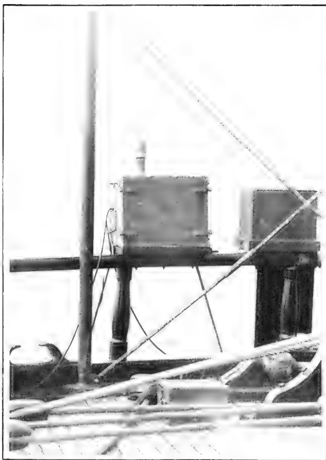
Fig. 16. View of short vertical collector rod on potential-gradient recording apparatus substituted for bent rod (fig. 11) on November 5, 1928
