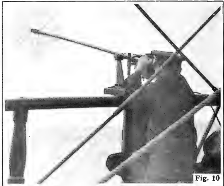
Fig. 8. Air-flow tubes of ion counter (small tube) and conductivity apparatus (large tube) on roof of atmospheric-electric cabin
