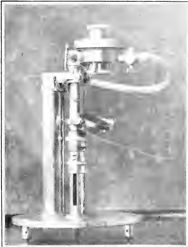
Fig. 13. Aitken nuclei counter, used to determine the number of condensation nuclei per cubic centimeter in the atmosphere
