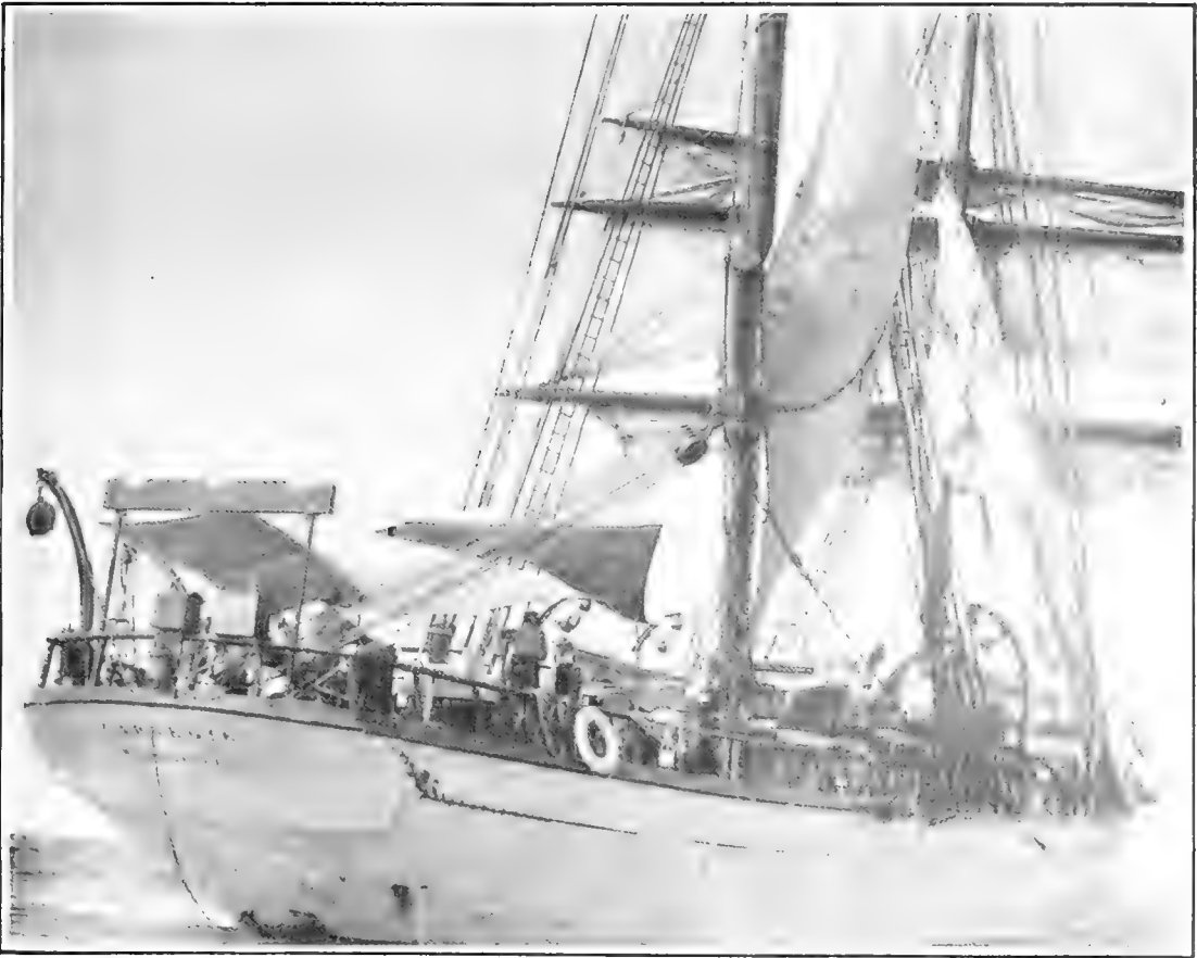
Fig. 18. View of potential-gradient recorder and eye-reading apparatus on stern rail of ship. Note how the boom crutch dominates the location, and shields the apparatus from distortion of the earth's field arising from the installation or removal of the quarter-deck awning. The mainsail is up with boom to starboard, a position designated as MUBS in this volume
