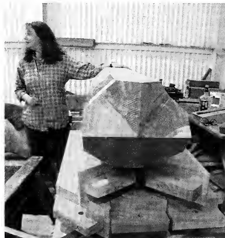
Stephanie (carpenter) with the kingpost for Waterston House (Bill Gardner)
