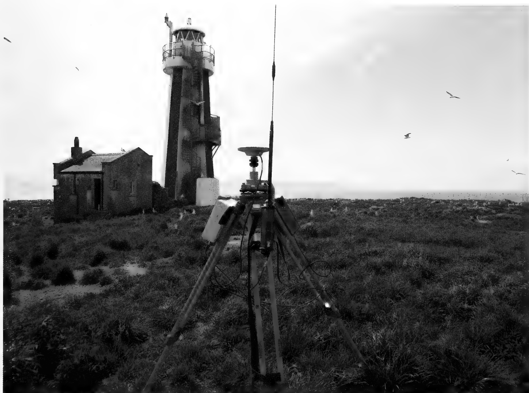
Plate 252. The Leica GPS base station was placed on the highest point of the island in order to provide the best signal with the mobile unit, Lady Isle, May 2012. © D. Grant
