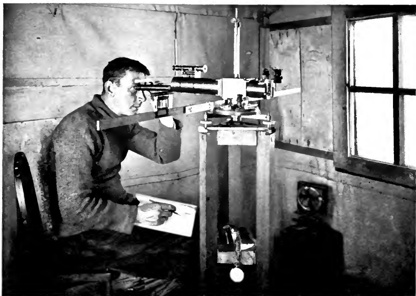
DR. SIMPSON AT THE UNIFILAR MAGNETOMETER
