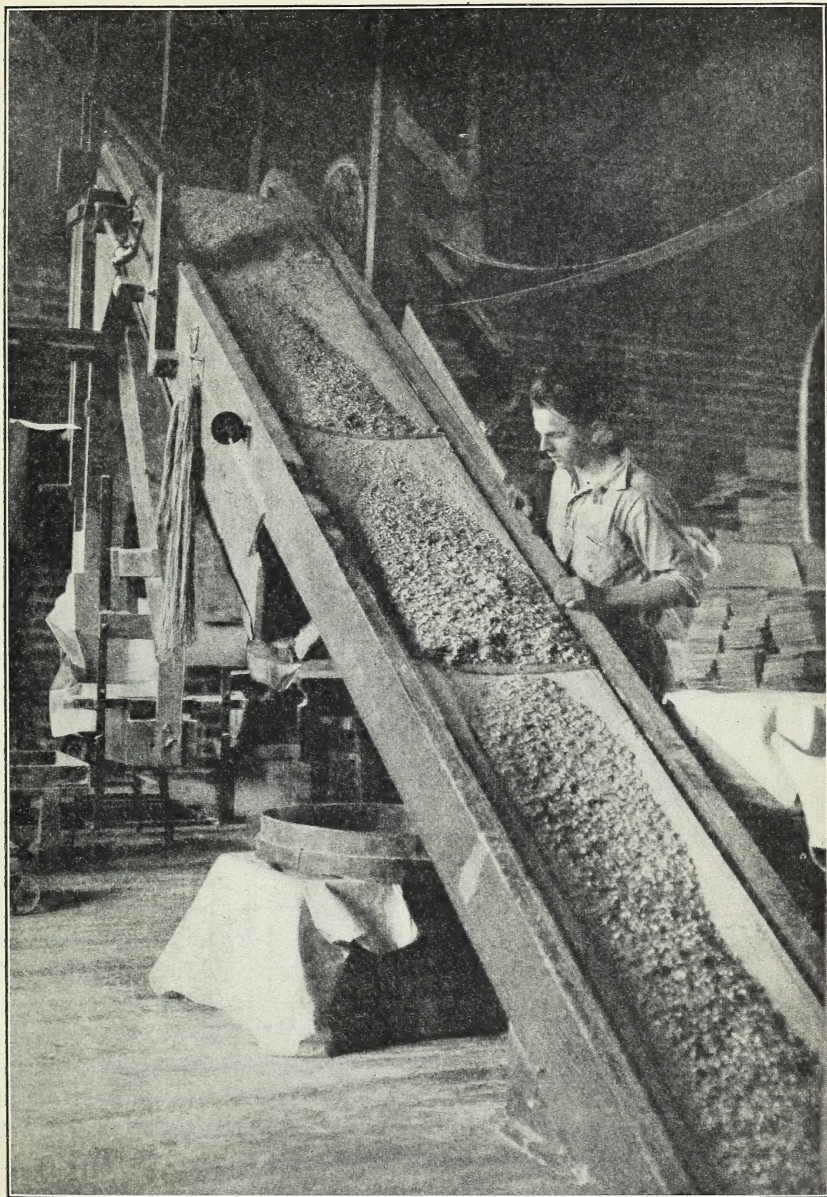
FIG. 5.—Cereal elevator which leads from sterilizer to packing room. Infestation may easily take place here. (Original.)
