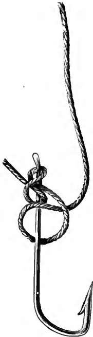
FIG. 26.—METHOD OF ATTACHING SNOOD TO FLATTENED HOOK
