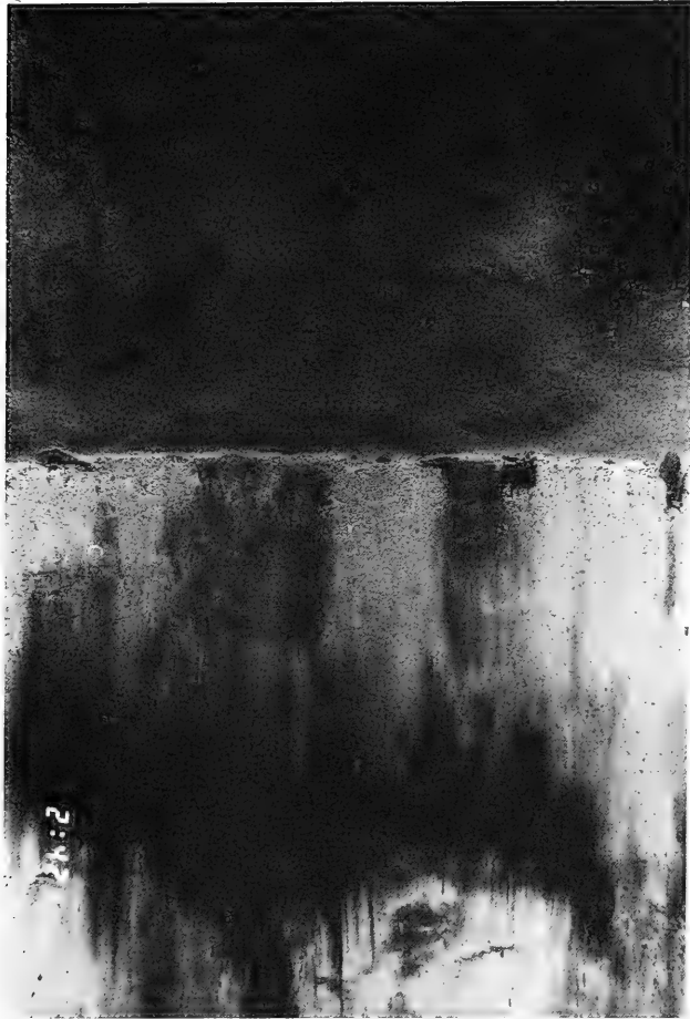
Figure 3-7. A REMOTS image from station 5-E showing a low-reflectance dredged material layer overlying a high-reflectance pre-disposal interface (arrow). Also note the patches of reduced (dark) sediment at the interface. Scale: Actual width of frame = 15.2cm.
