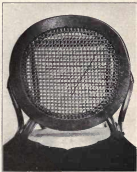
FIG. 25. FIRST DIAGONAL COMPLETED AND THE SECOND BEGUN. THE SIXTH STEP.
