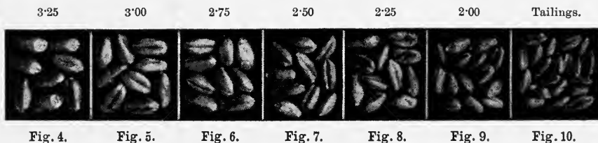
Figures showing the actual size of the grains belonging to each grade yielded by the sieves shown in Figures 2 and 3. The proper grade numbers are placed above each illustration.
