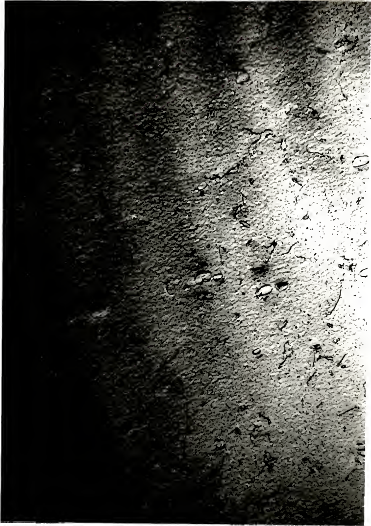
Fig. 37. Large dislocation loops observed in the thicker regions of the Al+100 ppm Cu sample (third dose). Analysis determined that these are interstitial loops of type \bar{n} = (011) , \bar{b} = a_0/2[011] . Magnification is 17,000.
