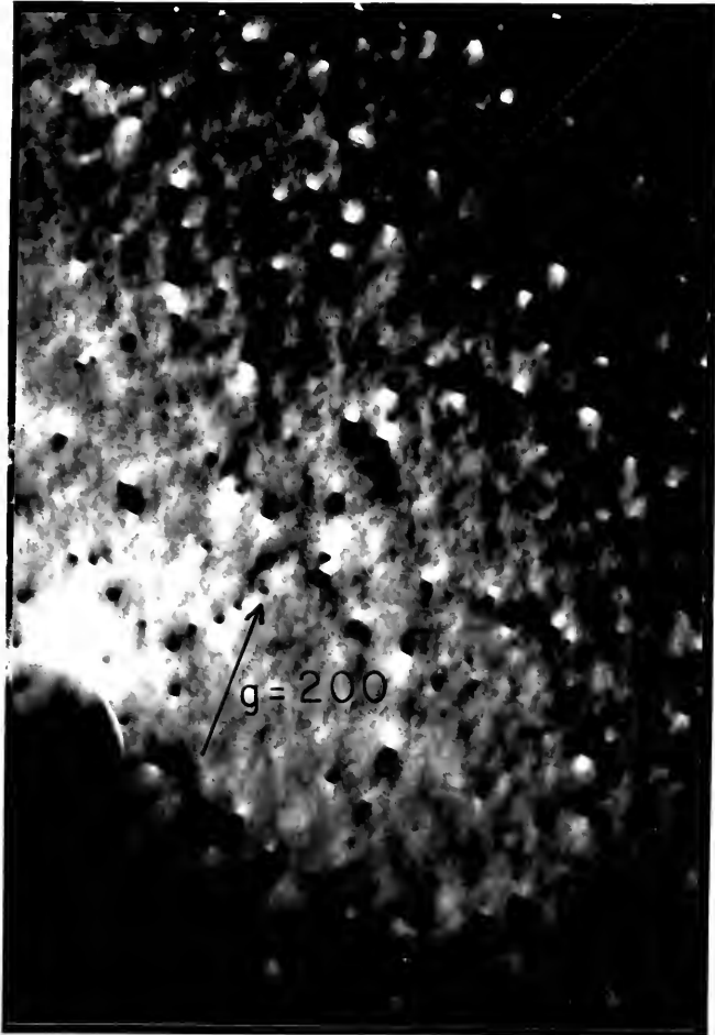
Fig. 34. Microstructure of the Al+100 ppm Cu alloy irradiated to the third neutron dose of 2 \times 10^{24} \text{ n/m}^2 (0.26 dpa). Magnification is 200,000.
