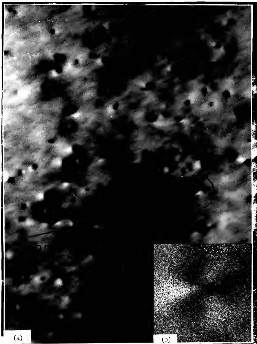
Fig. 27. Dislocation loops observed in electron irradiated (200 keV) pure aluminum (99.9999%). (a) \bar{z} = [0111] , \bar{g} = (200) and magnification is 250,000. (b) \bar{z} = [1121] , \bar{g} = (2\bar{2}0) and magnification is 2,000,000.
