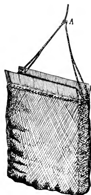
A marine dredge ready for use. Note the manner of fastening the two arms together at A, so that they will fall apart when an extra strain is brought upon them.
