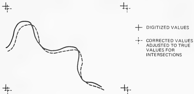
Figure 19. Digitization procedure for correcting shoreline position locations when original shoreline movement map distortions exist (Everts, Battley, and Gibson 1983)
