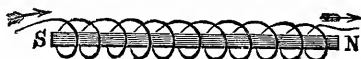
Coil of Electrified Copper Wire turning a Steel Bar into a Magnet.
