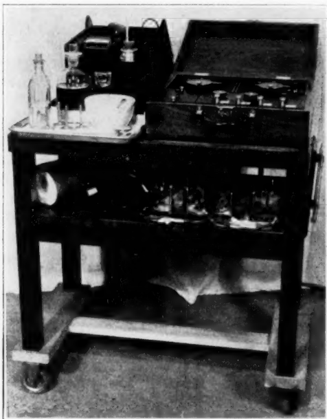
Fig. 2.—The dermohmeter, portable skin temperature apparatus, electrodes, electrode stands, paste and wet and dry bulb thermometers mounted on the carriage at the bedside.
