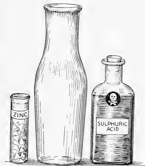
FIG. 4.—Apparatus used in preparing hydrogen.
