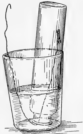
FIG. 3.—Apparatus used in preparing nitrogen.
