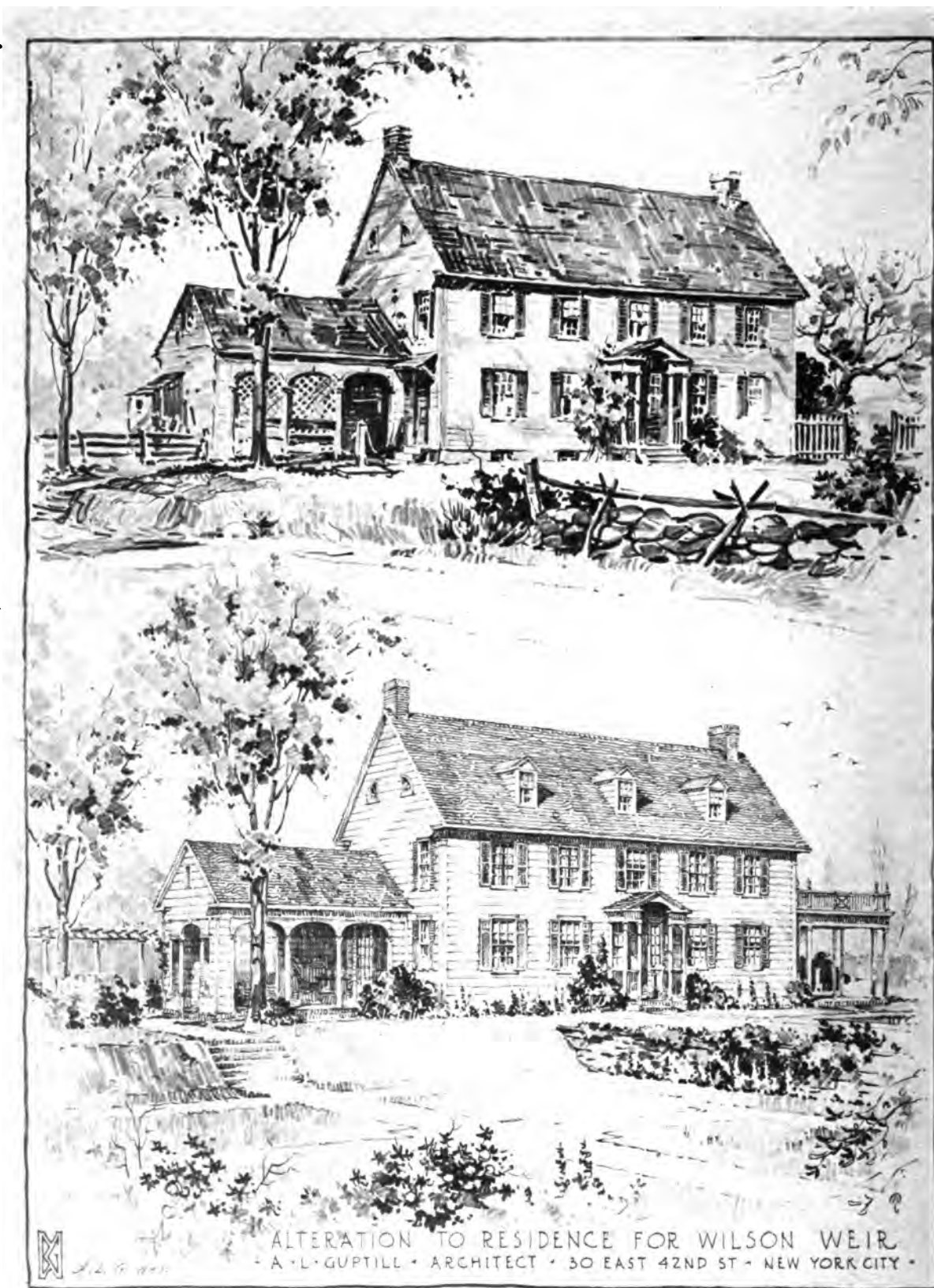
Figure 18. The Same Subject Drawn with Broad Lines and with Fine Lines. A Type of Sketch to be Submitted by the Architect to His Client to Show Proposed Alterations.
