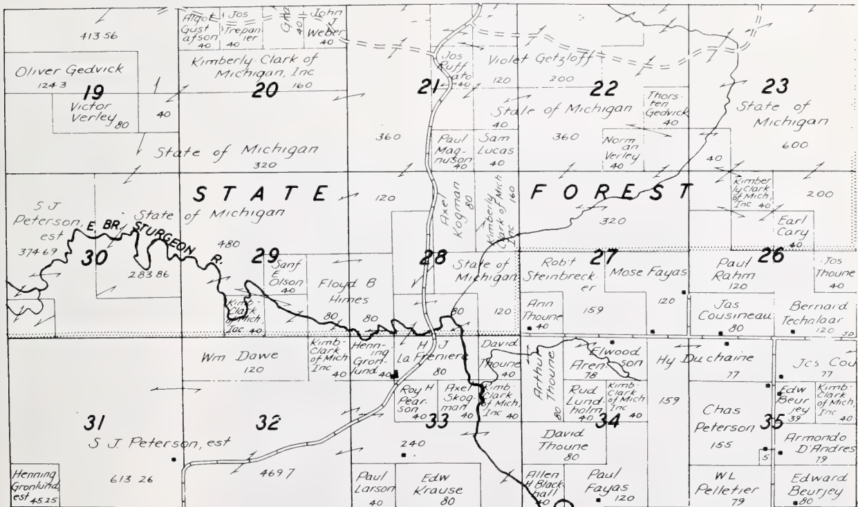
Figure 4.—To determine forest acreage owned, property descriptions of sample owners were first located on plat records such as this, and then the corresponding descriptions were examined stereoscopically on aerial photographs.
