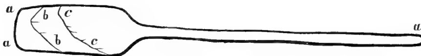
WOODEN SHOVEL, 3½ feet long—Waterbury Mine.— aa . Original form.— bb . Partially worn.— cc . Worn obliquely.
