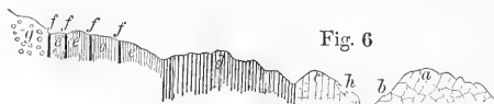
a. Granite. b. Fine-grained micaceous rock. c. Sandstone altered to quartzite. d. Limestone. e. Black clay-shale with four seams f of anthracite. g. Quartzose conglomerate. h. Creek alluvion.
