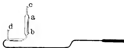
FIG. 39.—Apparatus for detecting absorption of oxygen by phosphorus pentoxide; filling with oxygen.
