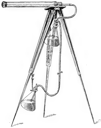
37.—Apparatus for counting microbes in the air.
