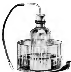
5.—Demonstration of carbonic acid in breath.
