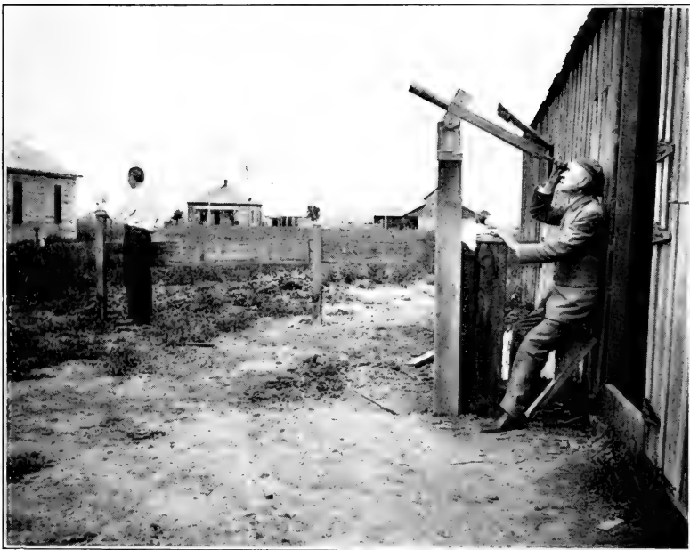
EXTERIOR OF OBSERVING SHELTER SHOWING POSITION OF PYRANOMETER AND VISUAL TELESCOPE.
