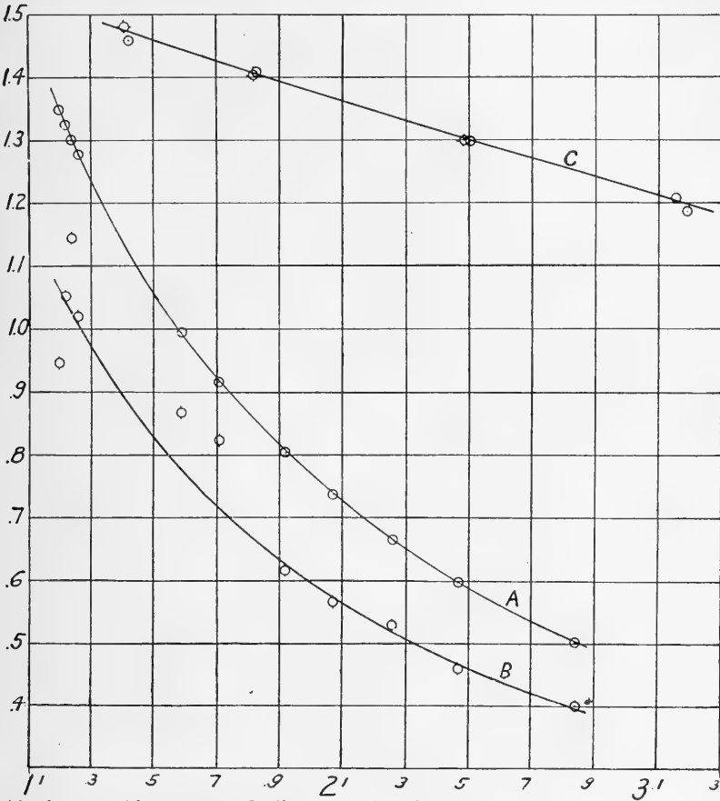
Abscissae = Air masses. Ordinates = Calories. Curve A = Total sky and sun per sq. cm. of horizontal surface. Curve B = Calories reflected from cloud per sq. cm. of horizontal surface. Curve C = Pyrheliometry of September 16, 1918. Total calories from sun alone per sq. cm. normal to beam.
