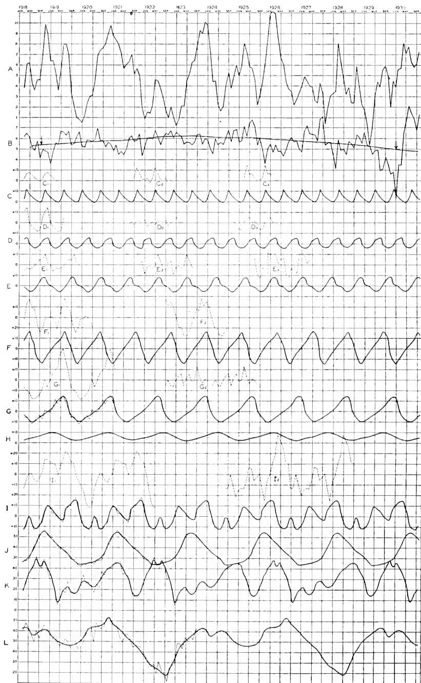
FIG. 6.—Temperature departures for Williston, N. Dak., and their periodicities. A, original data; C, 7-month; D, 8-month; E, 11-month; F, 13\frac{1}{2} -month; G, 18-month; H, 21-month; I, 25-month; J, 28-month; K, 45-month; L, 68-month; B, residual after removing periodicities, doubtfully showing 11 \frac{1}{4} -year periodicity.
