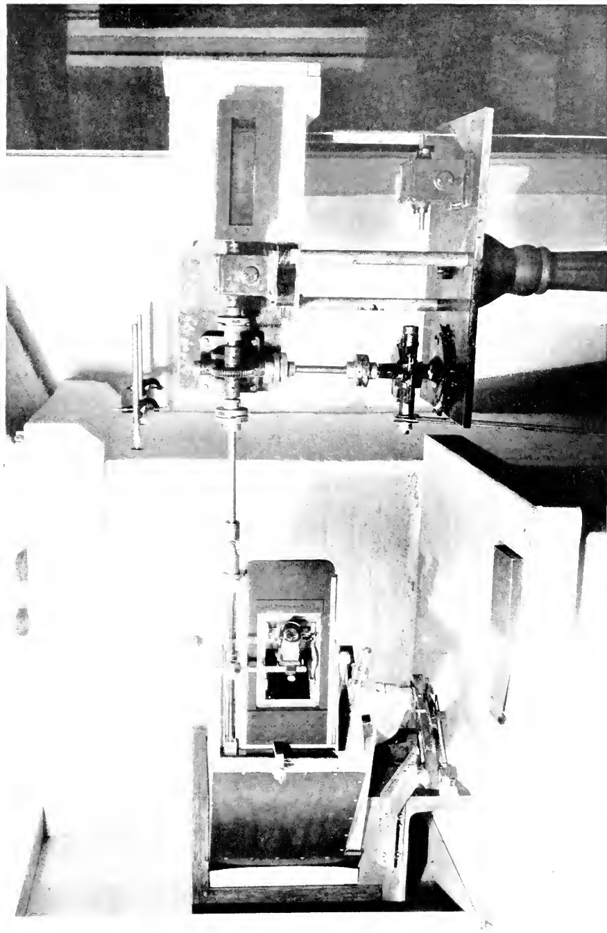
Camera of spectrograph showing mechanism for moving thermocouple and directly recording the spectrum.
