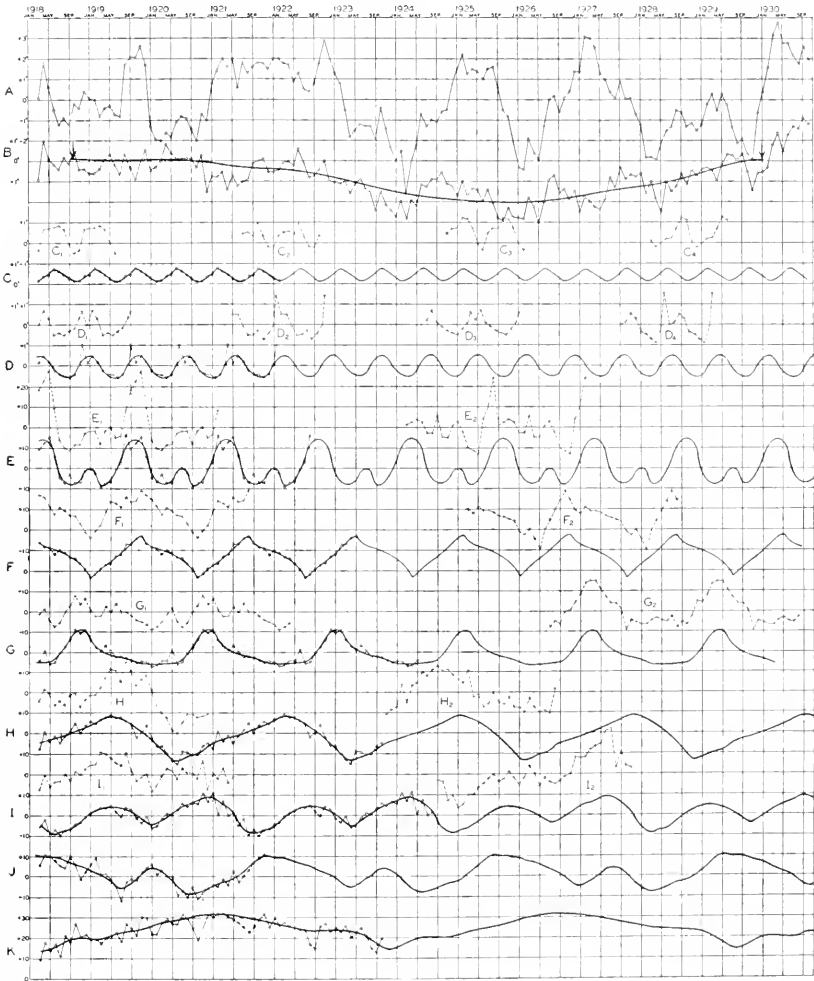
FIG. 4.—Temperature departures, Clanton, Ala., and their periodicities. A, original data; C, 8-month; D, 9½-month; E, 18-month; F, 21-month; G, 25-month; H, 34-month; I, 39-month; J, 45-month; K, 68-month; B, residual after removing periodicities, shows 11¼-year periodicity.
