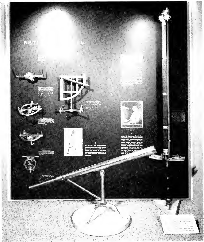
Hall of physical sciences: Instruments used to lay out the Nation's Capital and for other precise surveying in the late 18th century. Some of these were used by Andrew Ellicott. On the right is the 6-foot zenith sector built by David Rittenhouse of Philadelphia, with additions by Ellicott. It was the most accurate scientific instrument built in this country in the 18th century.
