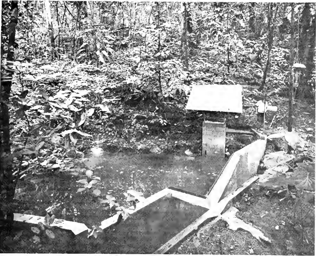
Large wier constructed on Barro Colorado Island by Environmental Science Program employees. Evapotranspiration, nutrient loss, and stream bed biota are being monitored.
