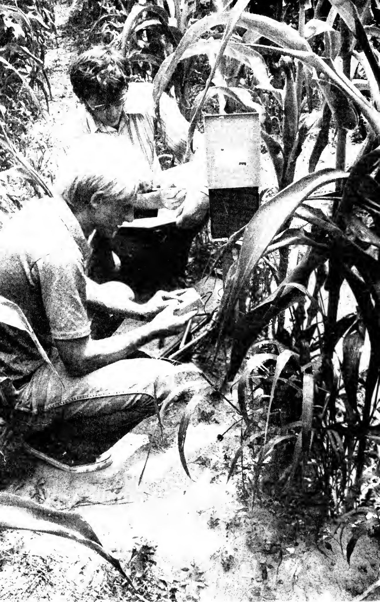
Two scientists at the Chesapeake Bay Center for Environmental Studies measure soil moisture as part of an investigation of the hydrologic characteristics of individual drainage basins.
