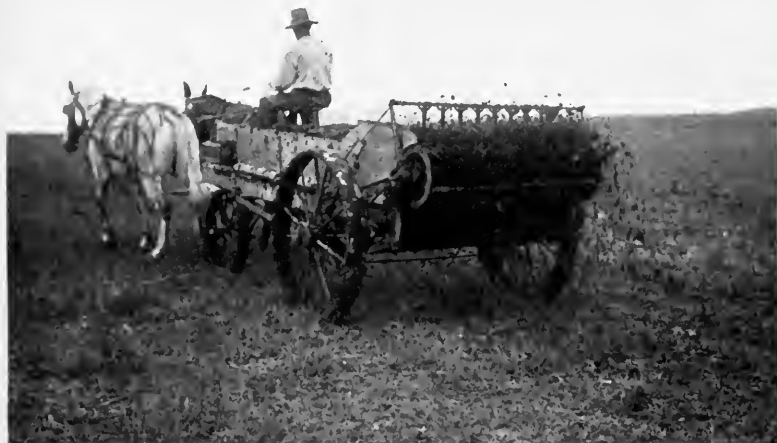
FIG. 83.—Manure spreader in action. The manure is torn apart so as to be scattered uniformly. (J. C. Beavers, Cir. 49 Purdue Station.)
