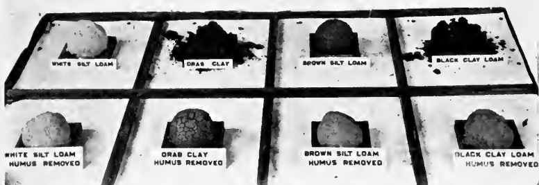
FIG. 78.—The effect of the removal of humus and of wetting and drying upon granulation. Drab clay is the only one that shows any tendency to granulate when humus is removed. (University of Illinois.)
