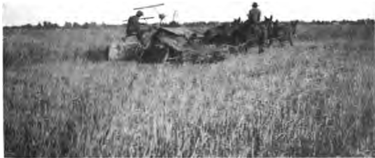
PLATE 22. —Cutting rice with a twine binder in the prairie rice district. The irrigation water was drained off the field a week or more before harvesting began. Heavy soil with a flat surface as in this field is ideal rice land. (Photo. from collection, Cereal Investigations, Bureau of Plant Industry.)
