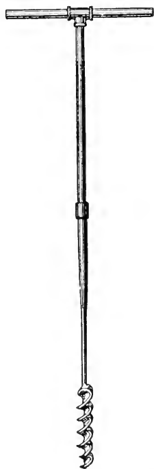
FIG. 3.—Soil Auger Made by Welding a Three-foot Length of Wrought Iron Gas-pipe onto the Shank of a 1\frac{1}{2} -inch Wood Auger. Additional lengths may be added as desired.
