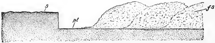
FIG. 11.—Land before and after plowing. The compactness of the soil is indicated by the density of dotting. Before plowing there is a compact surface crust (s), below which the soil becomes less and less compact as we go deeper. After plowing we find the soil (fs, furrow-slice) converted into a loose mass of crumbs (flocules), with increase of bulk. Compacted plow-sole at pl
