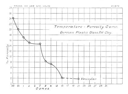
The foregoing curves show that there is a great difference in the behavior of various flint fire clays, and a sharp contrast between the behavior of flint clays and plastic clays.
