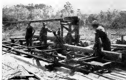
FIGURE 38.—Portable sawmill cutting shortleaf pine on the piedmont, capacity 6 M board feet a day.
