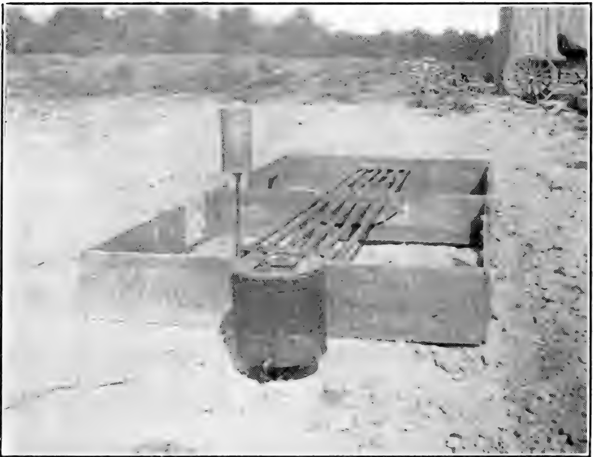
FIG. 12.—Showing frame, pipe system and heater tank of hot water brooder.
