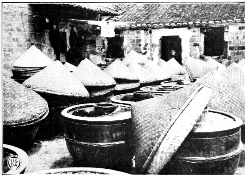
FIG. 2.—Ripening of soy sauce mash in Ichang, Hupe, China. "In the center of the large jars, full of fermented soy beans and brine, strong small baskets have been placed, in which the soy sauce accumulates and is dipped out, ready for use. This method of obtaining the soy sauce is possibly local." (Reproduced from a photograph taken in 1917 by F. N. Meyer.)
