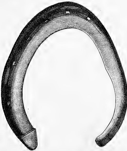
FIG. 14.—Ground surface of shoe shown in the previous figure. The inner nailless branch has the thickness of the outer branch plus its calk, so that the inner and outer quarters of the hoof are equidistant from the ground.
