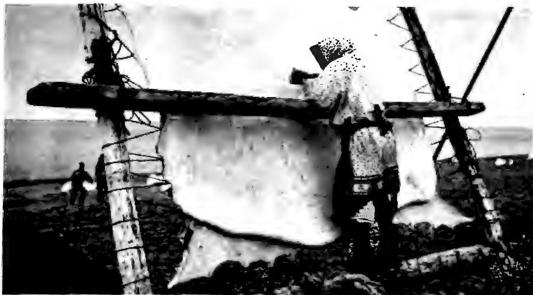
Figure 5.--Eskimo woman at Gambell splitting walrus hide for use as a boat covering. (Photo by Thayer)
