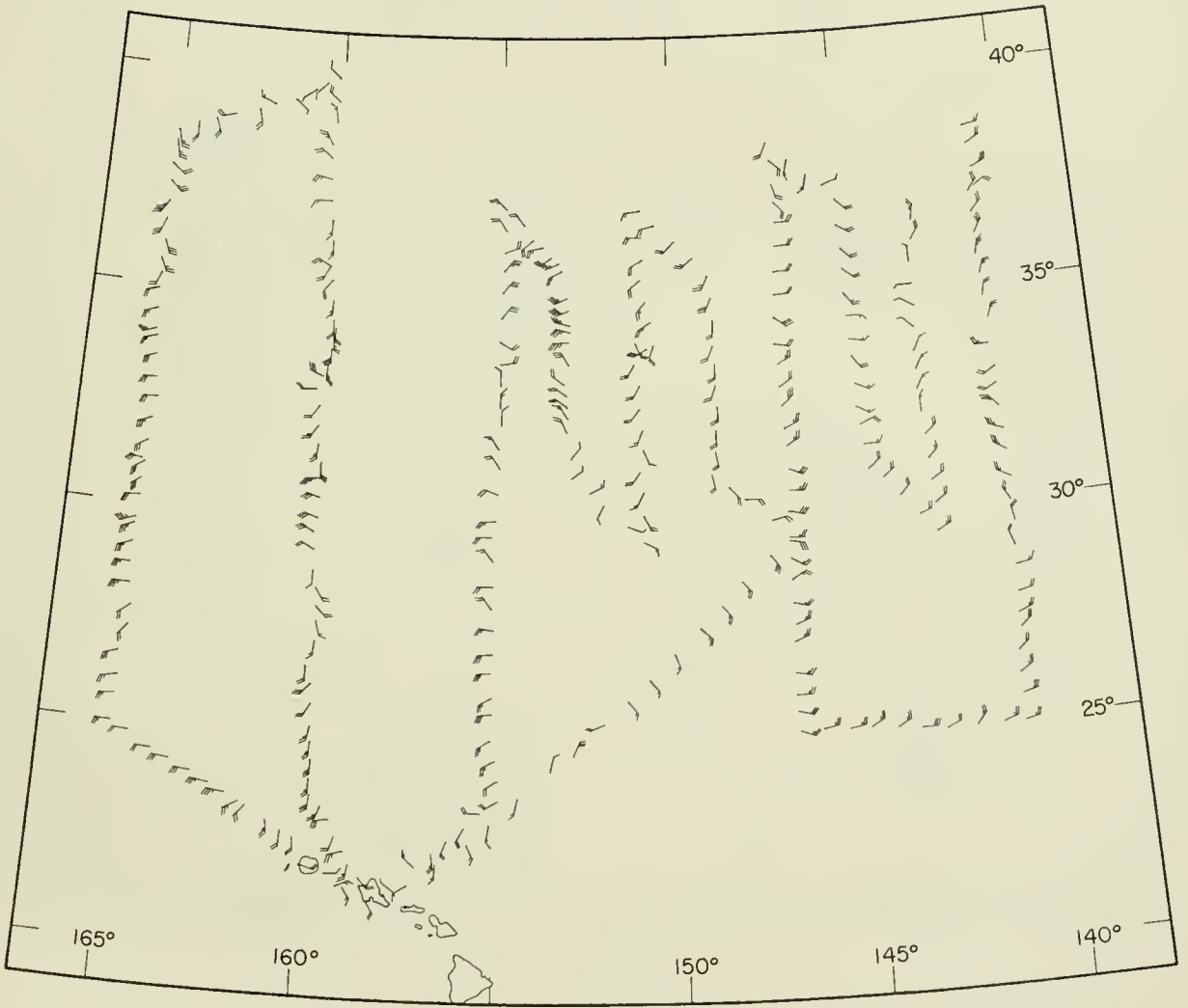
Figure 5.--Wind data taken at bathythermograph lowerings. Arrows point in direction of wind; given in Beaufort force, e.g., 1 long and 1 short barb indicates a Beaufort force 3 wind.
