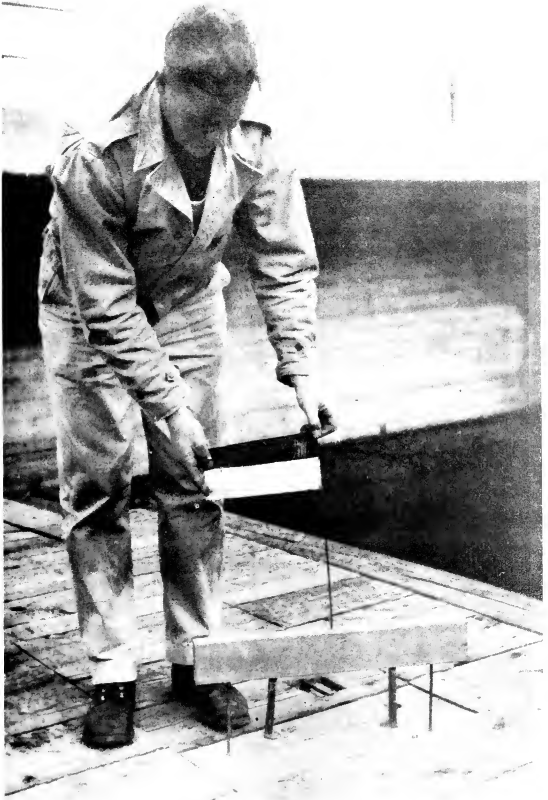
Figure 6.--Wooden float used in experiment to determine direction and influence of wind drift below Bonneville Dam.
