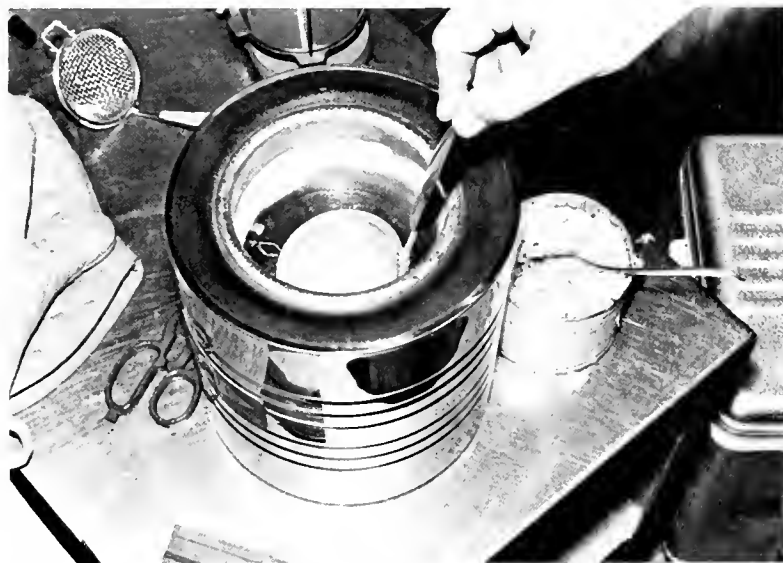
Figure I-2.—Immersion freezing of crab meat in food grade Freon 12.
